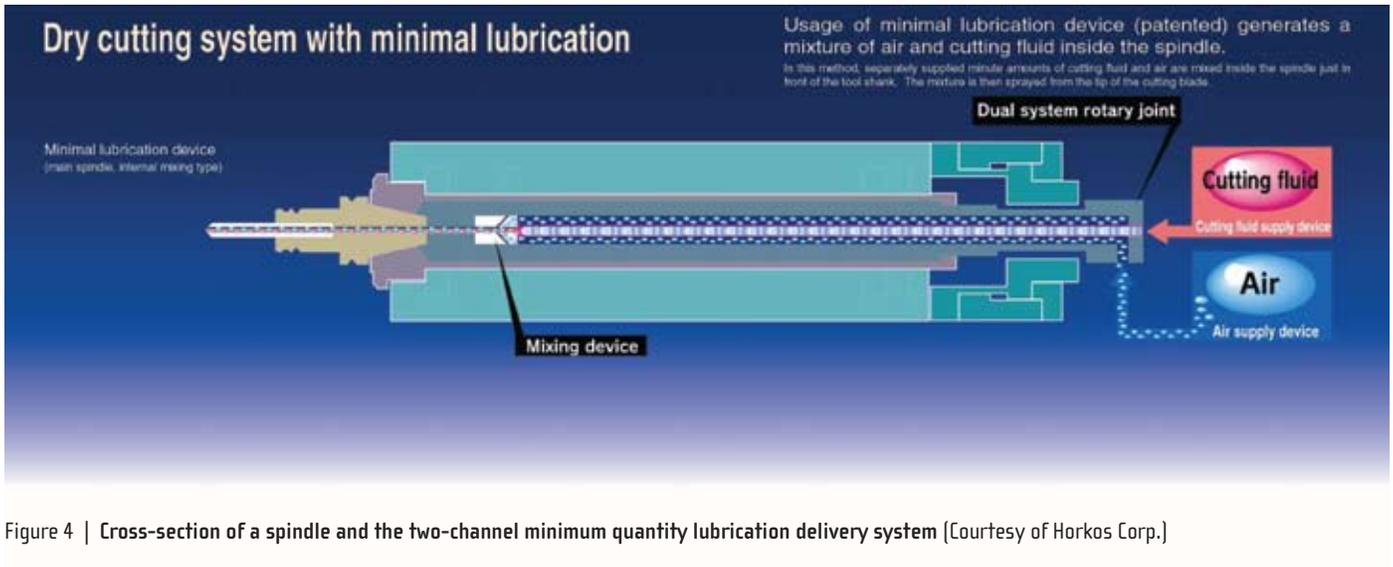
Figure 4 | Cross-section of a spindle and the two-channel minimum quantity lubrication delivery system (Courtesy of Horkos Corp.)
