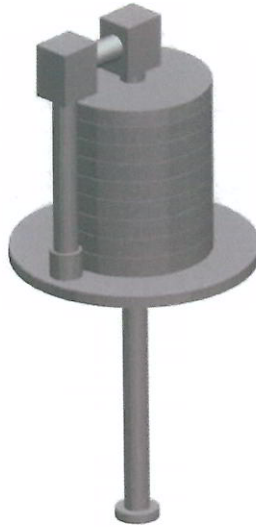
Fig. 1: CVD reactor for experimental studies as schematic representation
